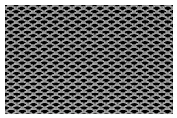
LW Pitch:10.00mmStrand Width:1.75mmSW Pitch:6.50mmThickness:1.50mmWeight:6.34 kg / m2Open Area:46%
